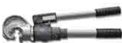
Hydraulic crimping tool Stocko WHPH 10 for the main contacts
