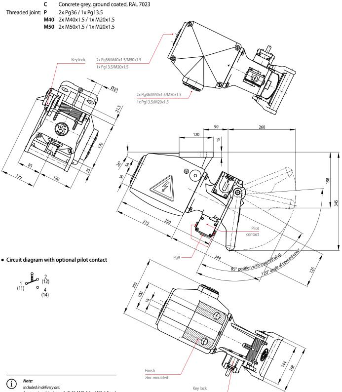
Included in delivery are: 2x screw-type blank caps 1x Pg36, M40x1.5 or M50x1.5 and 1x Pg13.5 or M20x1.5
