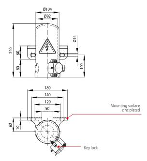
• ZH092 BD-V0-x Dummy without lock and key
